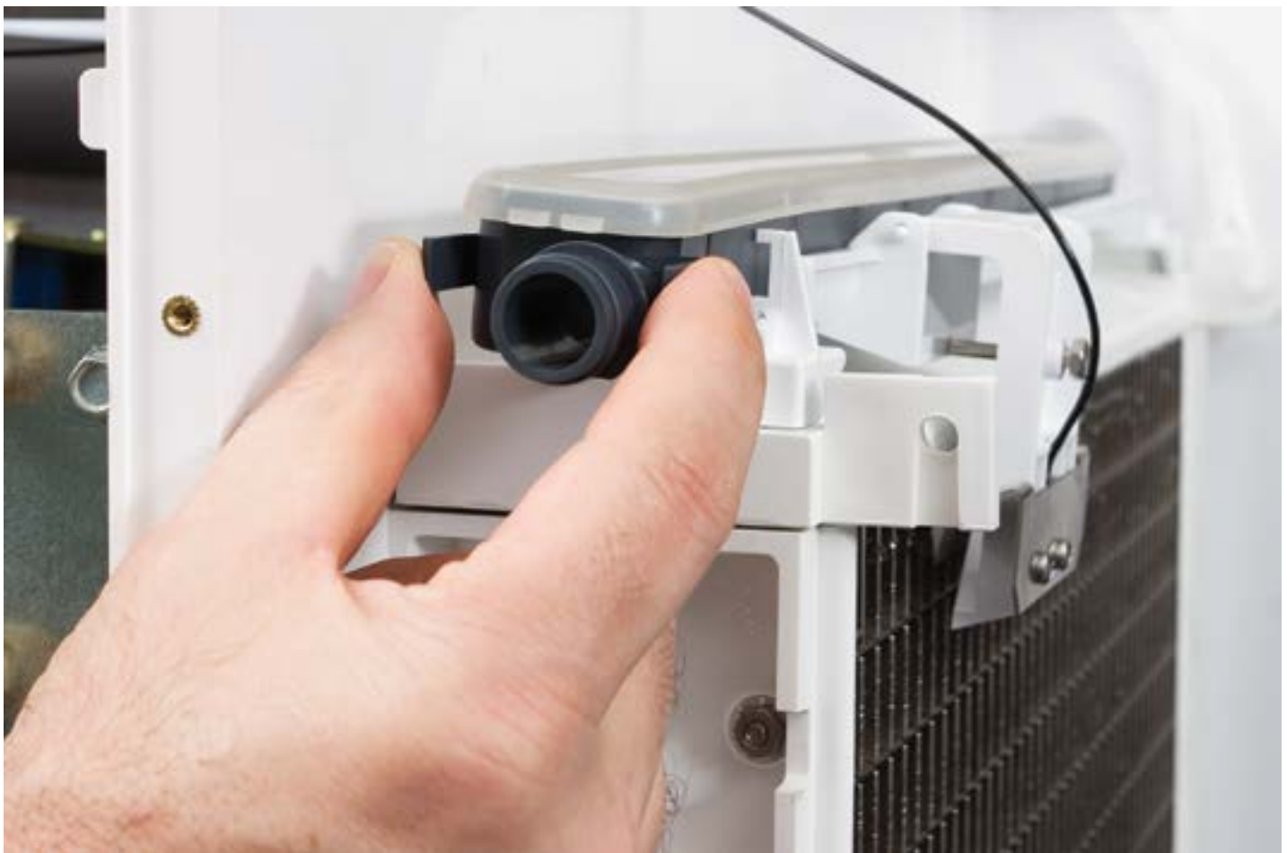
Water Distributor Removal
